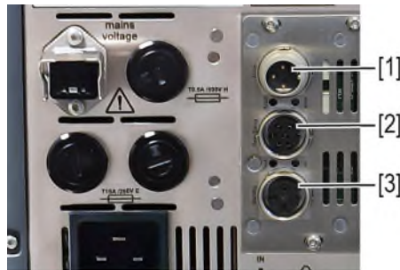
Slot with analogue connections
